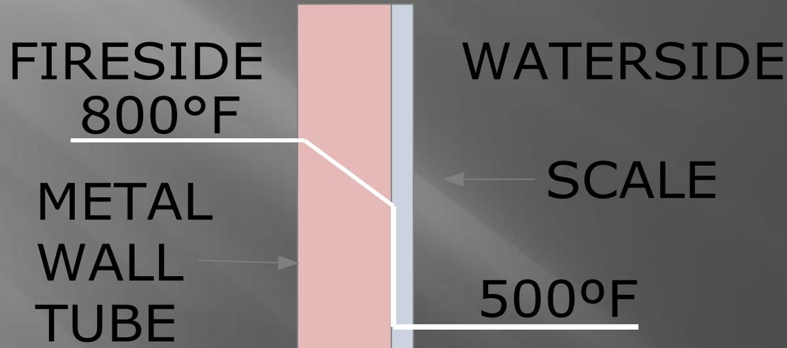
With the presence of scale, there exists a  $300^{\circ}\text{F}$  heat loss through the tube.
