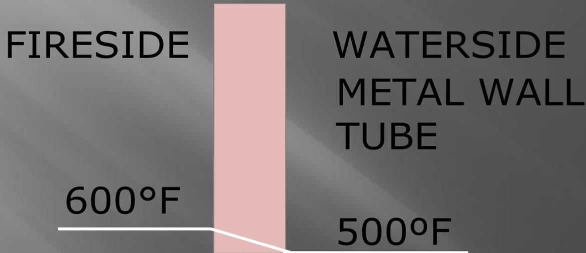
With no scale present, there exists only a  $100^{\circ}\text{F}$  heat loss through the tube.
