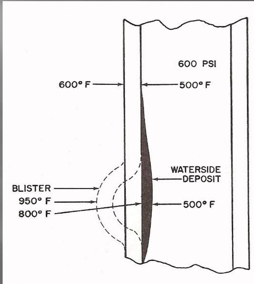
Effects of waterside deposits on boiler tubes.
